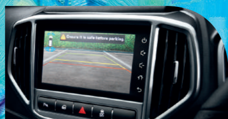
Reverse Camera with Dynamic Lines***
