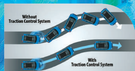
Electronic Control System (ESC) & Traction Control System (TCS)
