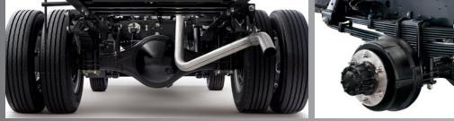
Longer leaf spring is sturdier, capable of handling heavier loads with less deflection for better driving comfort.
