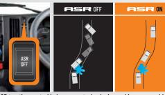
ASR traction control helps prevent wheelspins and improves vehicle EBD is a function that uses the ABS to distribute braking force between stability when driving on slippery roads.
