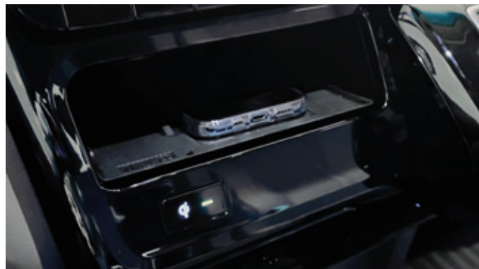
Wireless smartphone charging system
