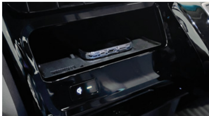
Wireless smartphone charging system*
