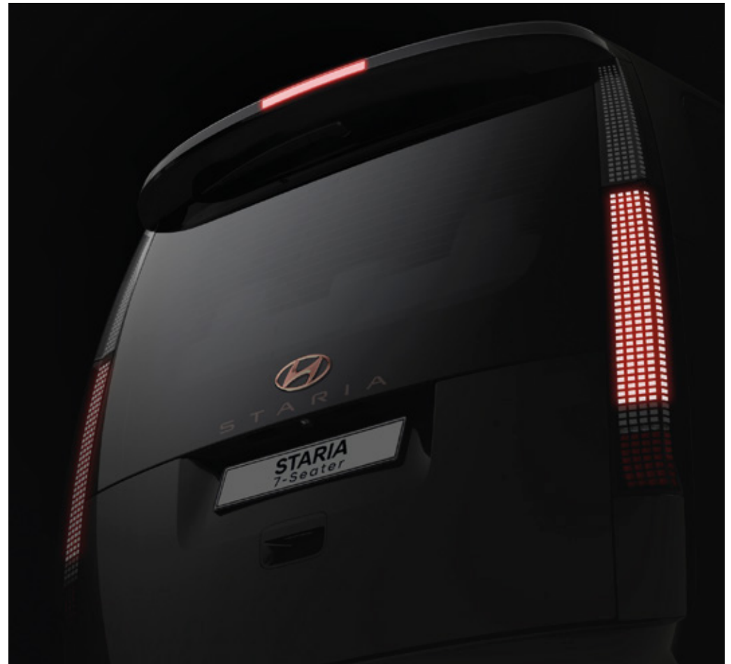
Parametric pixel lights (LED rear combination lamp)
