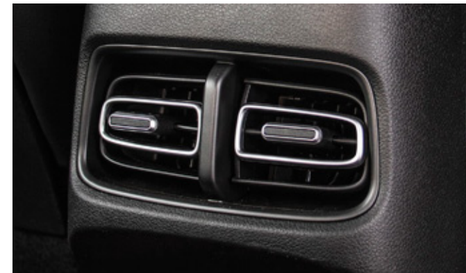
Rear air-cond vents
