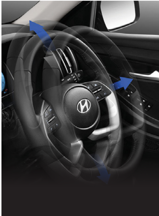
Tilt- and telescopically-adjustable steering wheel
