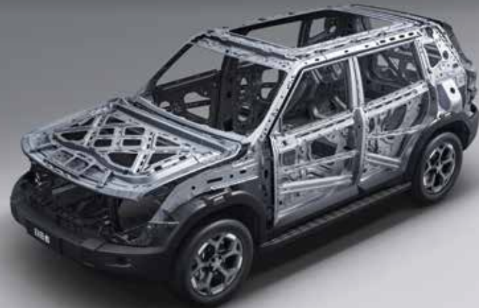
Reinforced Body Structure
